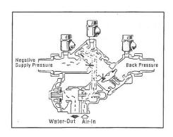
Leakage from a backflow preventer is normally attributed to foreign matter lodging on the seating area of either the first or second check valve. Most times this can be corrected by simply flushing the valve which will dislodge any loose particles. It is, therefore, most important on new installations that the piping be thoroughly flushed before installing the unit. It should be remembered, however, that spillage does not provide a "warning signal" that the valve is in need of maintenance.
